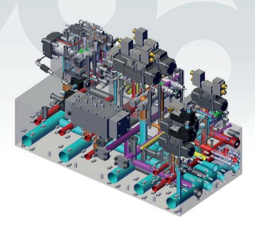
Starting from customer specifications, Oleobi designs and manufactures integrated manifolds. Prior to delivery each manifold is fully tested and certified to guarantee high performance and 100% safety for the operators.
